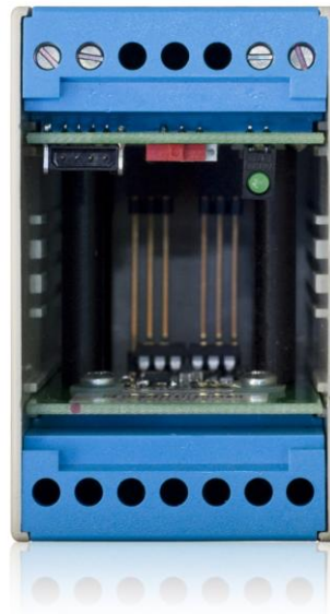
Photograph 2 Access to console port and programming switch
