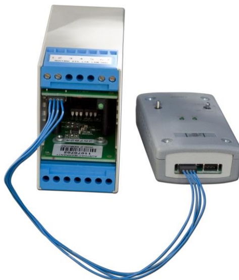
Photograph 3 Laptop connected to console port via MEAN1 interface
