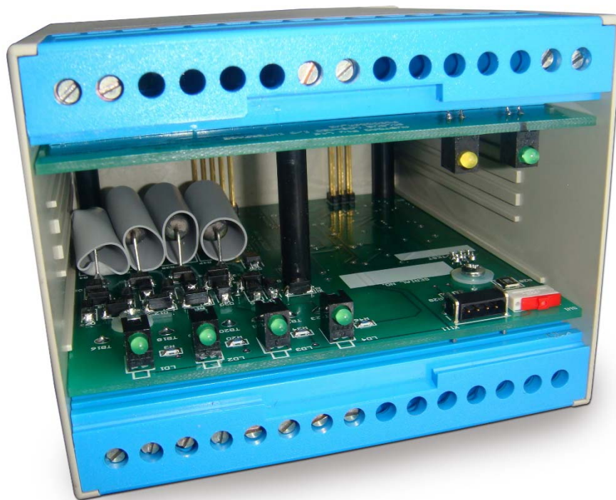
Photograph 2 Access to console port and programming switch
