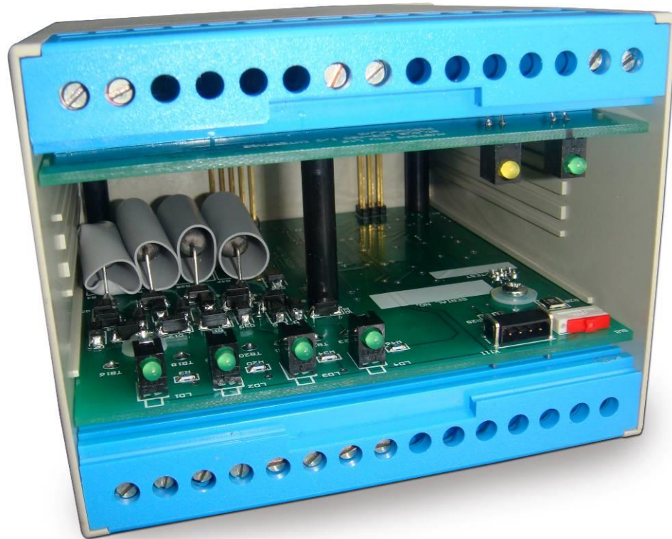
Photograph 2 Access to console port and programming switch
