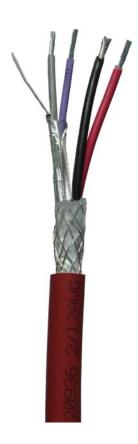
The 2.5mm<sup>2</sup> pairs are screened using a foil tape and a 24/0.2 TC drain conductor.
