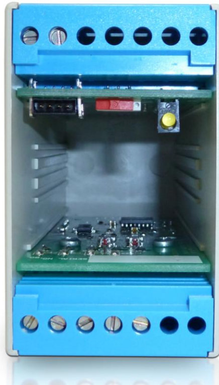
Photograph 2 Access to console port and programming switch
