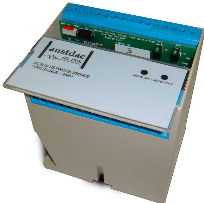
Photograph 2 Access to console ports and programming switches
