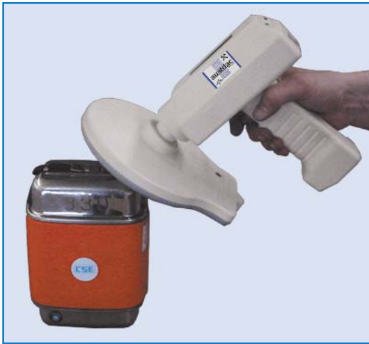
AusTran scanner testing self rescuer
