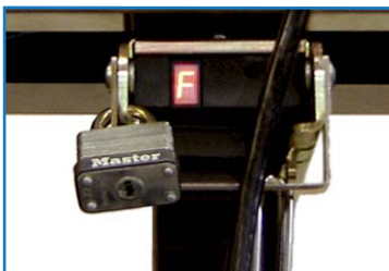
Fully Charged Lamp on Charging Rack with Lock
