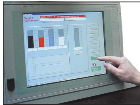
Computer Interface linking to the SILBUS underground network
